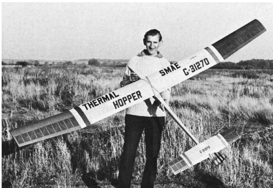
The ship rises smoothly on the line, holds on the hook till opportunity knocks. It's moderate size for soaring, practical to tote around, handle in the wind. Plug-in panels, follows proven concept.
